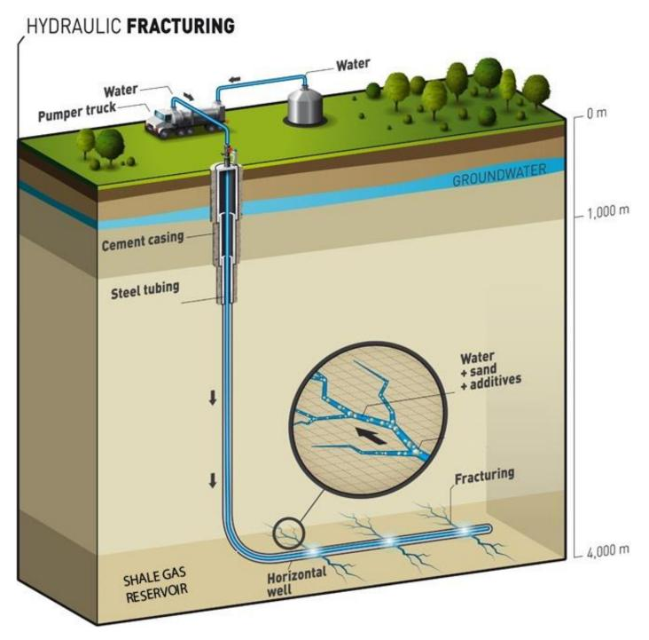
Figure 3: Schematic diagram of shale gas extraction process. Source: Modified from Total S.A.
