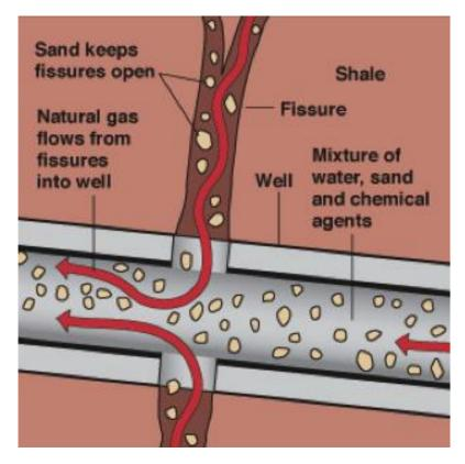
Figure 5: Diagram of proppant in action. Source: Modified from Al Granberg.
