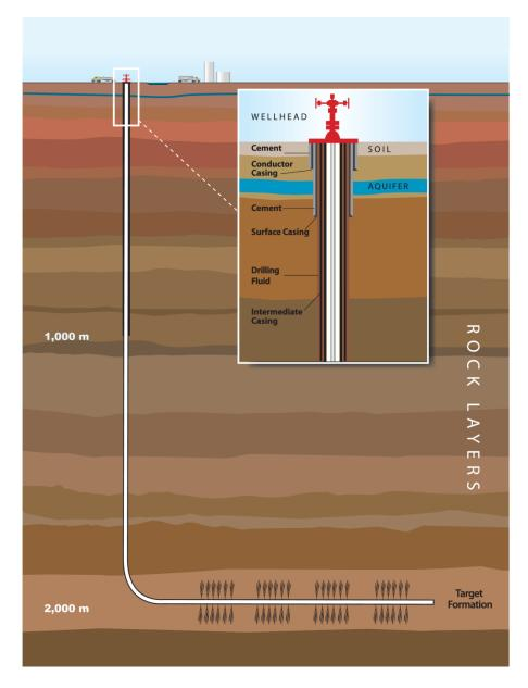
Figure 2: Schematic diagram showing typical well construction, casing, and horizontal drilling. Source: Modified from Society of Manufacturing Engineers.
